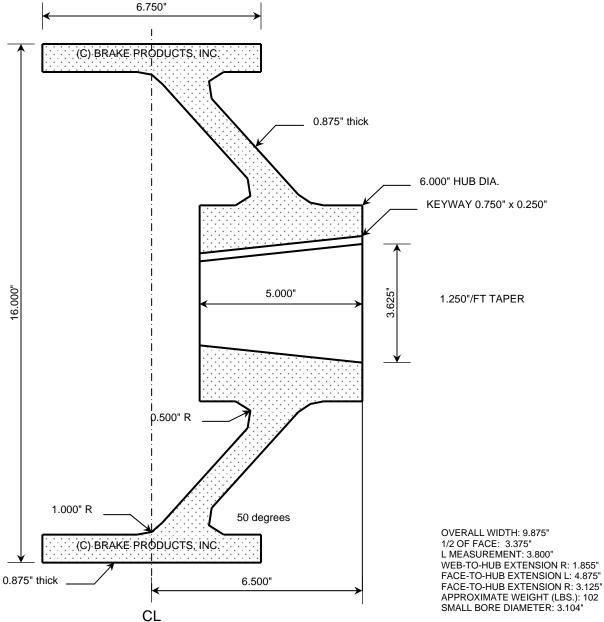
TOLERANCES: WHEEL DIAMETER: +0.005"/-0.000" BORE TAPER: +0.000"/-0.003"
